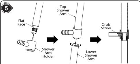
Assemble the **Top Shower Arm** into the **Shower Arm Holder**, note that the **Top Shower Arm** can only be assembled one way, so ensure that the flat faces of **Top Shower Arm** and **Shower Arm Holder** are aligned.
