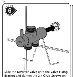
Note: Do not fully tighten the screws as some adjustment of the valve will be necessary when assembling the **Shower Arms**.
